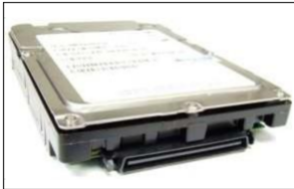
c. SCSI (Small Computer System Interface)
